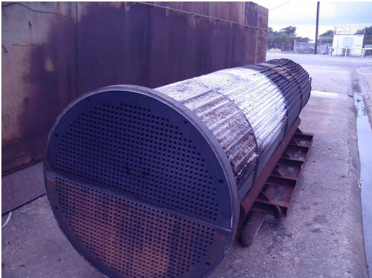
Figure 12. Polymer found on methyl acetylene removal tower reboiler bundle pulled on or around September 10, 2019. (Credit: TPC)
